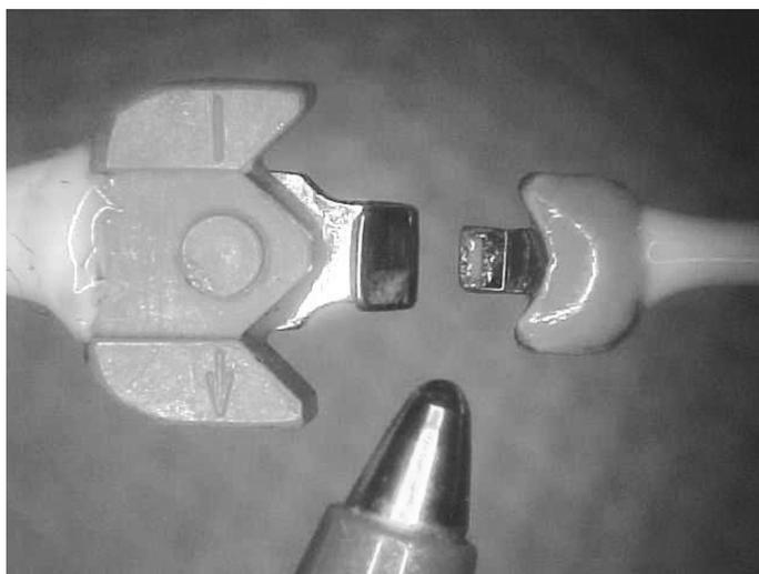
Figure 2: Ballpoint pen tip vs. assembled SU-8 flowprobe (right) and the smallest flowprobe prior to Nanofab research (left).
